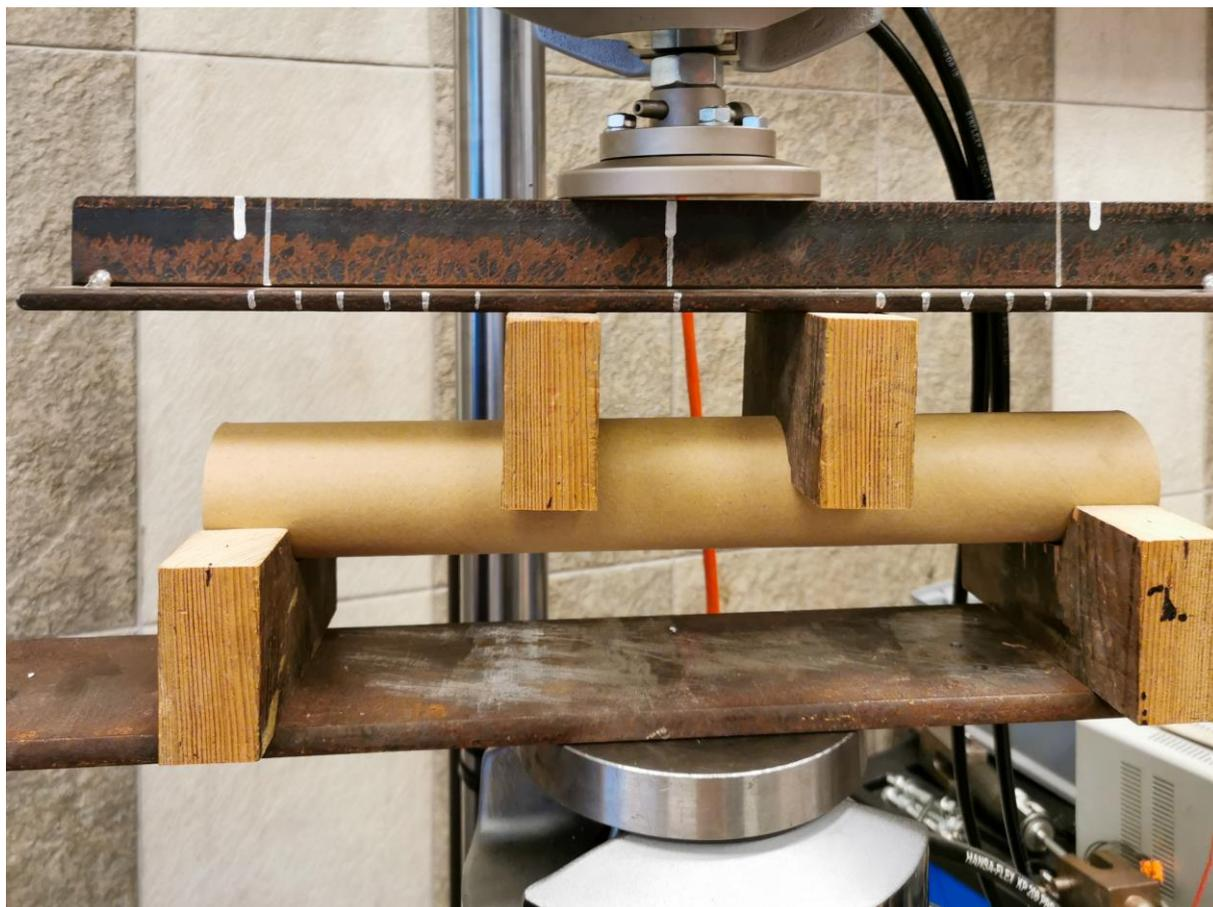
Fig. 1. Structural tests on paper tube
