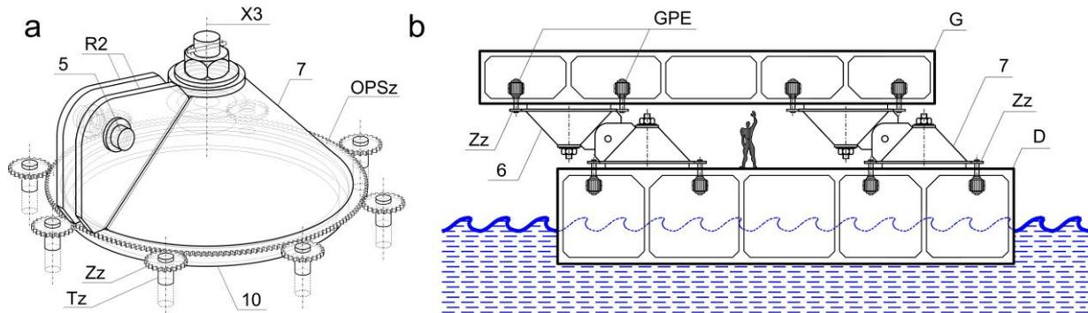
Fig. 2. a) View of the conical body equipped with a rack and pinion stabilizing ring (OPSz), b) vertical section of a floating platform designed as a power station.
